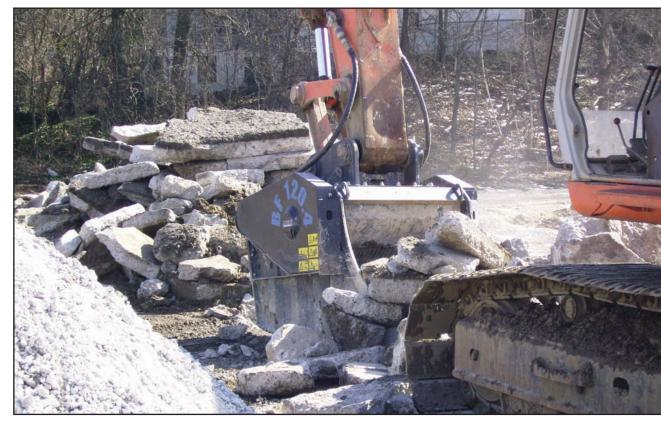
The BF120 is the largest in a line of five models, it mounts on excavators 68,000 pounds and up and has a 1.25 cubic yard capacity.
